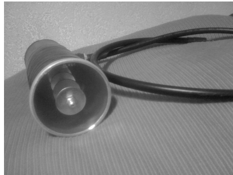
Figure 2: The Yagi Pringles antenna
